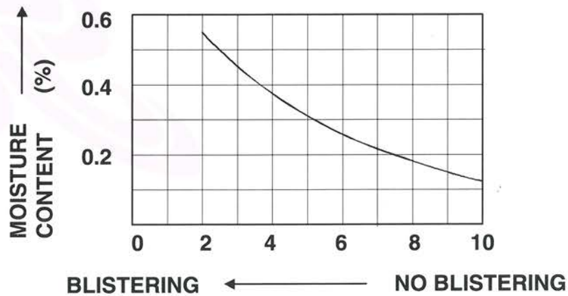
Fig. 6.4: Effect of moisture content on intensity of blistering for high-impact polystyrene.
